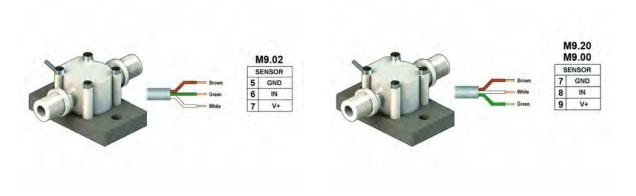
Wiring connections of ULFXX.H to the other monitors
